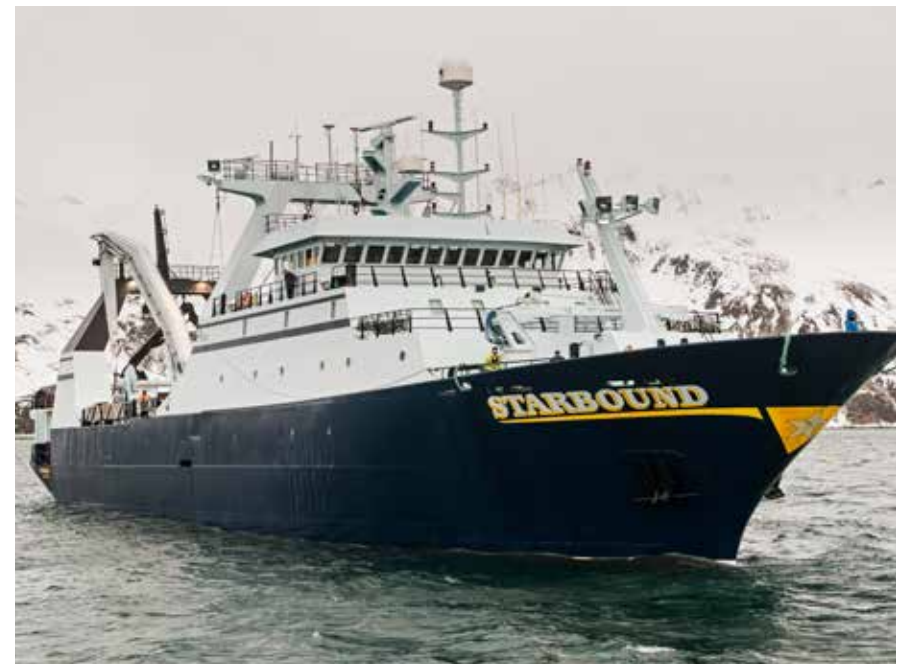
The C/P Starbound is one of 17 AFA Catcher Processors vessels operating in the Bering Sea. AFA CPs primarily target pollock and can have crews of 100 or more. The Starbound was lengthened 60' in 2015 to accommodate a fish meal plant and other upgrades.
